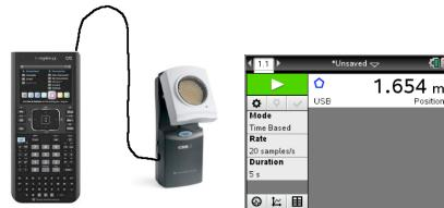
Now make sure the device is set to collect data for 10 seconds by clicking on the **Duration** menu and setting it to 10 seconds. Since we want to see the graph produced as your group member walks, click on the graph tab at the lower left corner of the window.
