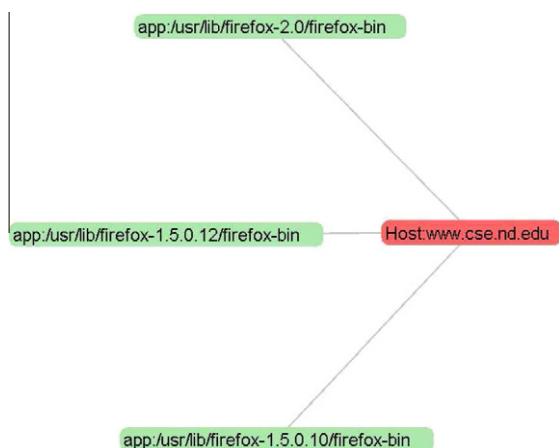
Fig. 9. A simple example showing policy compliance control on application versions for vulnerability avoidance and license management.
