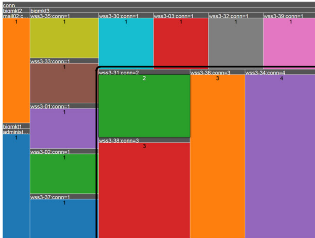
Figure 8. Hierarchical rectangles in the treemaps' view may represent properties of servers or workstations in subnets. The area size of rectangles can be used to visualize machines' status, for example, in this case, larger sizes suggest possible anomalous connectivity status of servers (highlighted).
