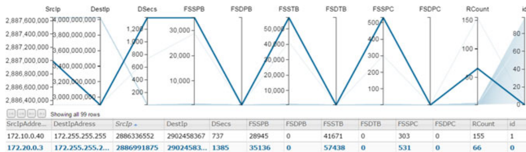
Figure 5. Attributes of network connections (edges) and their anomalies can be visually examined in detail from parallel coordinate system. Each individual connection (e.g., 172.20.0.3→172.255.255.255) may be highlighted by selection in the bottom table.
