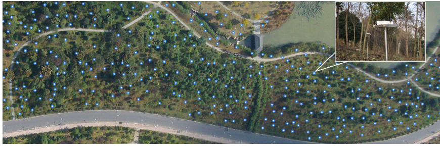
Figure 2: The bird's-eye view of the GreenOrbs deployment in Zhejiang Forestry University. The latest deployment includes 500 physical sensor nodes in total. A portion of the sensor nodes have been in continuous operation for over one year.
