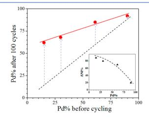
**Figure 6.** Comparison of changes in composition of  $Pd_nNi_{100-n}/C$  catalysts before and after 100 potential cycles from 1.2 to 0.02 V at a scan rate of 50 mV/s in N<sub>2</sub>-saturated 0.1 M HClO<sub>4</sub> solution. (inset) Loss of Ni in the catalysts ( $\Delta$ Ni%) after potential cycling, calculated assuming Ni is the only leaching species.
