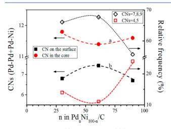
**Figure 8.** CNs in the core (a) and on the surface (b) (left vertical axis for closed circles and squares), and the relative frequencies corresponding to the CNs on the surface (right vertical axis for open diamonds and squares). The frequencies are in terms of high (CN = 7, 8, and 9) and low (CN = 4 and 5) coordinated surface atoms in Pd<sub>n</sub>Ni<sub>100-n</sub> NPs for Pd atoms.
