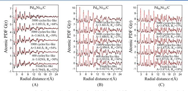
**Figure 9.** Ex-situ atomic PDFs data for  $Pd_nNi_{100-n}/C$  catalysts after accelerated durability test with different potential cycle numbers (potential cycling in 0.1 M HClO<sub>4</sub> under N<sub>2</sub> between 0.4–1.0 V vs RHE at 50 mV/s) where n = 30 (A), 61 (B), and 90 (C). The potential cycling numbers are indicated for each curve. Experimental data are given as symbols and model data as lines. Models are based on an fcc-type structure.
