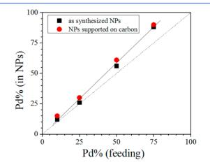
**Figure 1.** Plot of Pd composition in Pd<sub>n</sub>Ni<sub>100-n</sub> nanoparticles (from ICP-OES analysis) vs the synthetic feeding composition. The dashed line represents a 1:1 relationship. The solid line represents the linear fitting to the NPs/C data (slope: 1.2,  $R^2 = 0.997$ ).
