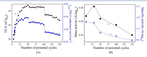
**Figure 5.** ECA and  $I_{\text{peak}}$  (Pd–O reduction) (A) and ORR mass activity and specific activity (B) as a function of potential cycles for Pd<sub>30</sub>Ni<sub>70</sub>/C (0.02–1.2 V vs RHE). Electrolyte: 0.1 M HClO<sub>4</sub> saturated with N<sub>2</sub> for determining ECA and 0.1 M HClO<sub>4</sub> saturated with O<sub>2</sub> for determining mass activity.
