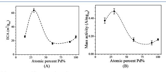
**Figure 4.** ECA (A) and mass activity (B) data at 0.8 V (vs RHE) for Pd/C, Pd<sub>15</sub>Ni<sub>85</sub>/C, Pd<sub>30</sub>Ni<sub>70</sub>/C, Pd<sub>61</sub>Ni<sub>39</sub>/C, and Pd<sub>90</sub>Ni<sub>10</sub>/C, as a function of Pd% in the bimetallic composition. Electrolyte: 0.1 M HClO<sub>4</sub> saturated with N<sub>2</sub> for determining ECA and 0.1 M HClO<sub>4</sub> saturated with O<sub>2</sub> for determining mass activity.
