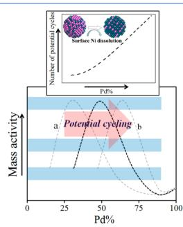
**Figure 11.** Dynamic illustration of the general trends observed for the mass activity vs bimetallic composition correlation for  $Pd_nNi_{100-n}/C$  catalysts before (curve a) and after extensive potential cycling (curve b). (top) Trend for the change in composition for  $Pd_{30}NI_{70}/C$  catalyst as a result of Ni-leaching during the potential cycling.
