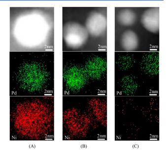
**Figure 2.** High-angle annular dark field scanning HAADF-STEM images (top panel) and elemental maps (middle and bottom panels) for  $Pd_{30}Ni_{70}/C$  (A),  $Pd_{61}Ni_{39}/C$  (B), and  $Pd_{90}Ni_{10}/C$  (C) nanoparticles (Ni species are in red and Pd species in green). The particle sizes are 7.1  $\pm$  1.1, 5.9  $\pm$  1.0, and 5.4  $\pm$  1.3 nm, respectively.
