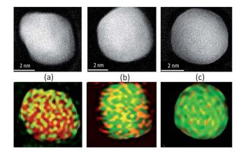
Fig. 6 HAADF-STEM images (up) and EELS elemental maps (down) for single  $Pd_xNi_{100-x}$  NPs with x=26 (a), x=56 (b) and x=88 (c). Elemental maps show rather scattered distribution of Pd and Ni species across the NPs reflecting their random-alloy character. Ni species distribution is in red and Pd species distribution is in green.
