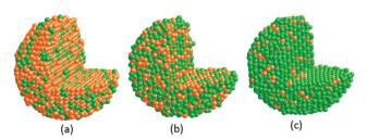
Fig. 4 Atomic structure solutions for  $Pd_xNi_{100-x}$  NPs (x=26 (a), 56 (b) and 88 (c)) as optimized by hybrid RMC simulations. The solutions feature 4100 atom configurations with local fcc-like ordering and random alloy chemical patterns. Atomic PDFs computed from the solutions are matched against the respective experimental PDFs in Fig. 5. Pd atoms are in green and Ni atoms are in orange.
