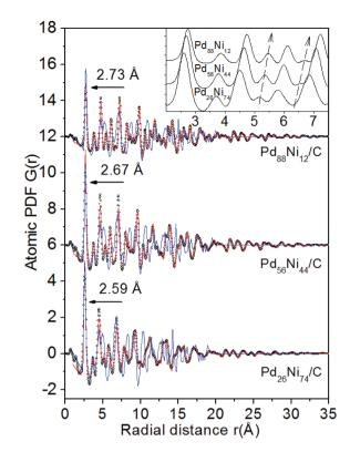
Fig. 1 Experimental (symbols), fcc-type crystallographic (lines in red) and icosahedral-type non-crystallographic (lines in blue) structure based PDFs for  $Pd_xNi_{100-x}$  NPs. The position of the first peak in each experimental PDF is marked with a solid horizontal arrow. The low-r part of the experimental PDFs (lines in black) is shown in the inset. Dashed arrows mark the evolution of subtle PDF features, i.e. of subtle structural features of  $Pd_xNi_{100-x}$  NPs, with Pd/Ni ratio.
