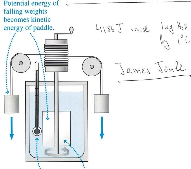
The paddle's kinetic energy in turn becomes internal energy of the water, indicated by rising temperature.
