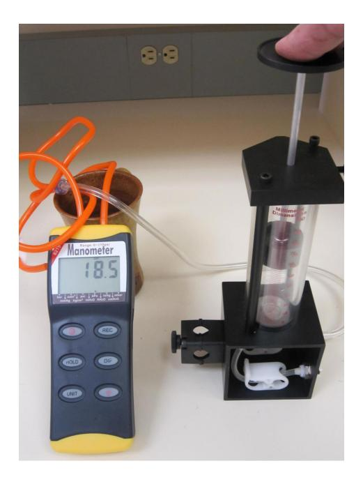
Record the height of the piston and the pressure when the platform is raised to its highest position. Press the platform down to a series of levels and record the height and pressure at each level. Convert the height measurements to gas volume measurements. Summarize the data with units in the respective data sheet below. For better precision run the manometer in "Differential pressure mode" (see Appendix 1 on page 10). Make a graph of gas pressure vs volume.
