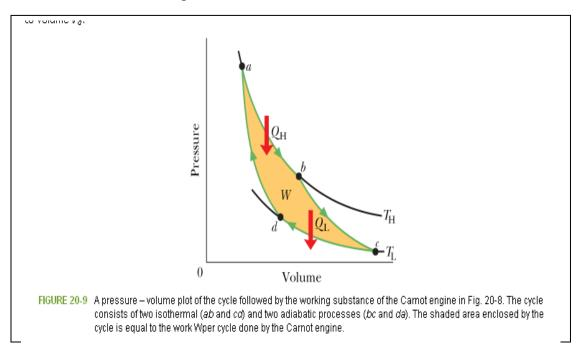
The **thermodynamic work**, *W*, per cycle can be estimated from the area enclosed by the respective cycle, e.g. the area enclosed by the polygon *abcd* in the P-V diagram above. Numerically W can be expressed as a function of the volume and pressure changes across the cycle *abcd* by the following expression:
