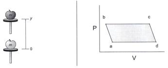
From that diagram estimate the thermodynamic work per cycle in joules and compare it with the useful mechanical work (left in the plot above) done in lifting the 200 g mass. Comment on the outcome of the comparison.
