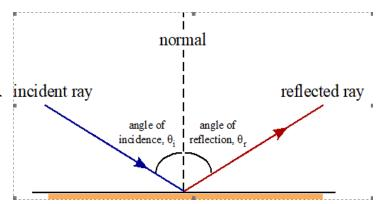
The angle of incidence is the angle between the normal and the incident ray; the angle of reflection is the angle between the normal and the reflected ray. The law of reflection states that the angle of incidence equals the angle of reflection:
