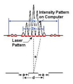
Figure 2: Double Slit Interference
