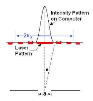
Figure 1: Single Slit Diffraction
