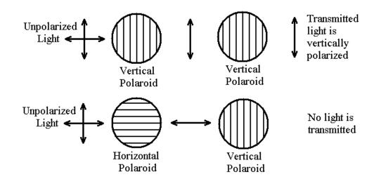
In the example shown, the two Polaroids are oriented at an angle  $\theta$  between  $0 \bullet$  and  $90 \bullet$ . Malus' Law tells us that if  $I_m$  is the intensity of the light transmitted when  $\theta$  is  $0 \bullet$ , then at any other angle the intensity of the light is  $I = I_m \cos^2 \theta$ .
