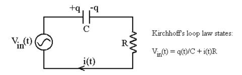
Since the capacitor represents an open circuit, the current i(t) is the rate at which the capacitor is charging.
