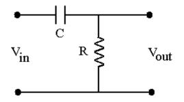
In this experiment, you will study the attenuation (decrease in amplitude) and phase shift of  $V_{out}$  relative to  $V_{in}$ . These two properties are referred to as the "frequency response" of the RC filter. The filter is called "high pass" because high frequency signals are not attenuated.
