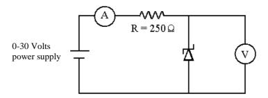
The maximum power rating of the 1N5346 is 1 watt and its Zener voltage is about 9 volts. Do not exceed the corresponding maximum current rating of (1 watt)/(9 volts) = 100 mA.
