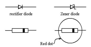
The factor which determines whether a diode is a rectifier or a Zener is the relative concentration of impurity atoms.
