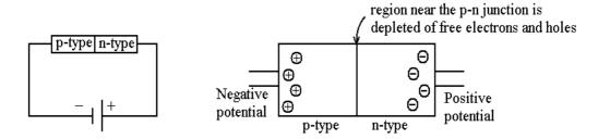
In this case the free electrons in the n-type region and the holes in the p-type region migrate away form the junction. Since there are few free electrons or holes near the junction, only a very small electric current flows and the diode is said to be reverse biased. Thus a semiconductor diode has the property that it conducts electric current in one direction and blocks the flow of current in the other direction.
