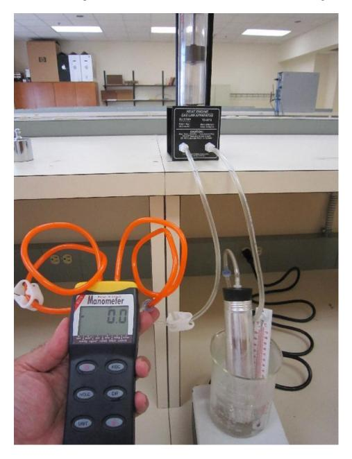
the top of the engine's platform. Remove the chamber from the beaker with cold water and place it in a beaker with boiling water (see the picture above). The temperature of the gas/air trapped inside the glass cylinder, hoses and air chamber will increase, causing the gas to expand and the platform to rise. The 200 g mass on the platform will rise
