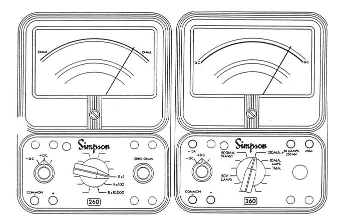
Jacks and switch positions for measuring resistance
