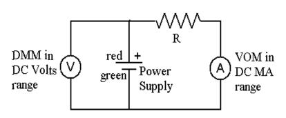
negative currents up to 1.5 mA. To obtain the negative values of current simply reverse the leads attached to the power supply.
