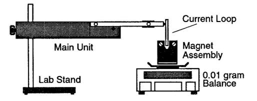
Turn the current on. If the reading is negative, reverse the leads where they plug into the arms of the Main Unit. The measured weight is directly proportional to the force caused by the current moving through the magnetic filed created by the Magnet Assembly.
