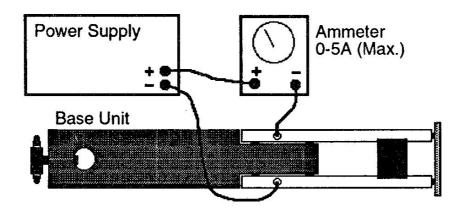
Place the long Magnet assembly on the balance and tare the reading by pressing the appropriate switch on it. This subtracts the weight of the Magnetic assembly, so only the force caused by the current will be measured.
