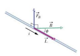
If a wire is not straight or the field is not uniform, we can imagine the wire broken up into small straight segments and apply the above equation to each segment. The force on the wire as a whole is then the vector sum of all the forces on the segments that make it up. In using the above equation bear in mind that there is no such thing as an isolated current-carrying wire segment of length L. There must be always a way to
