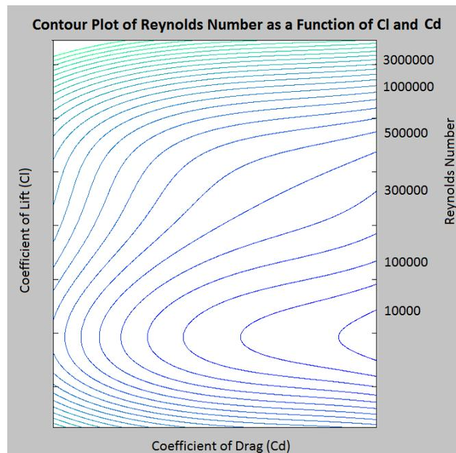
Figure 5 – Contour Plot of the 3-D surface interpolation analytically relating coefficients of lift, coefficient of drag, and Reynolds Number.
