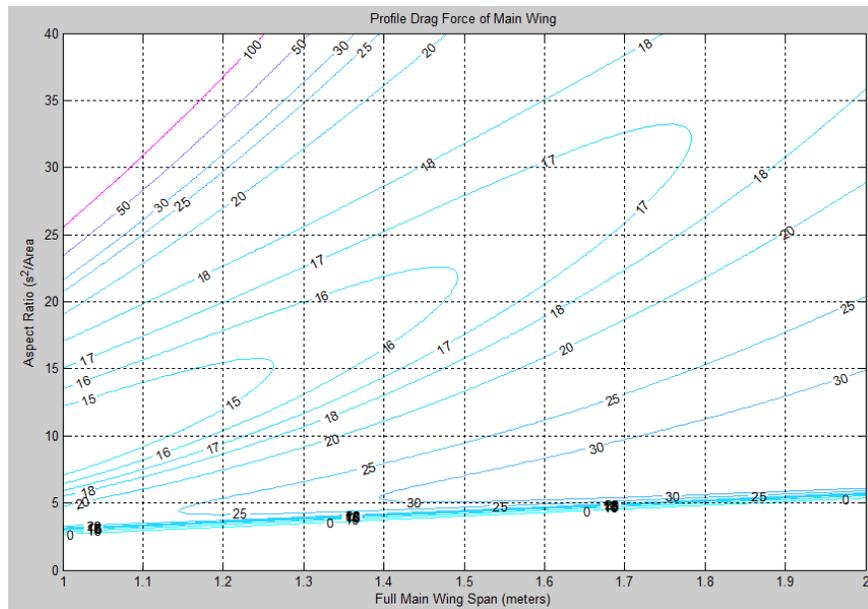
Figure 6. Contour Plot of the Profile Drag Force as a Function of Span and Aspect Ratio.
