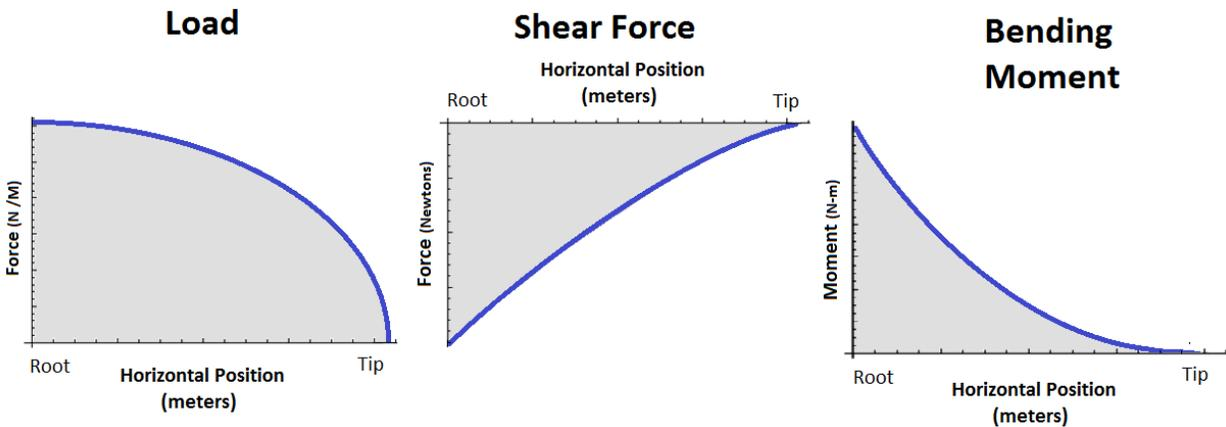
*Figure 8 – Load, Shear and Bending Moment Diagrams for an elliptic distribution of lift on a cantilevered wing.*
