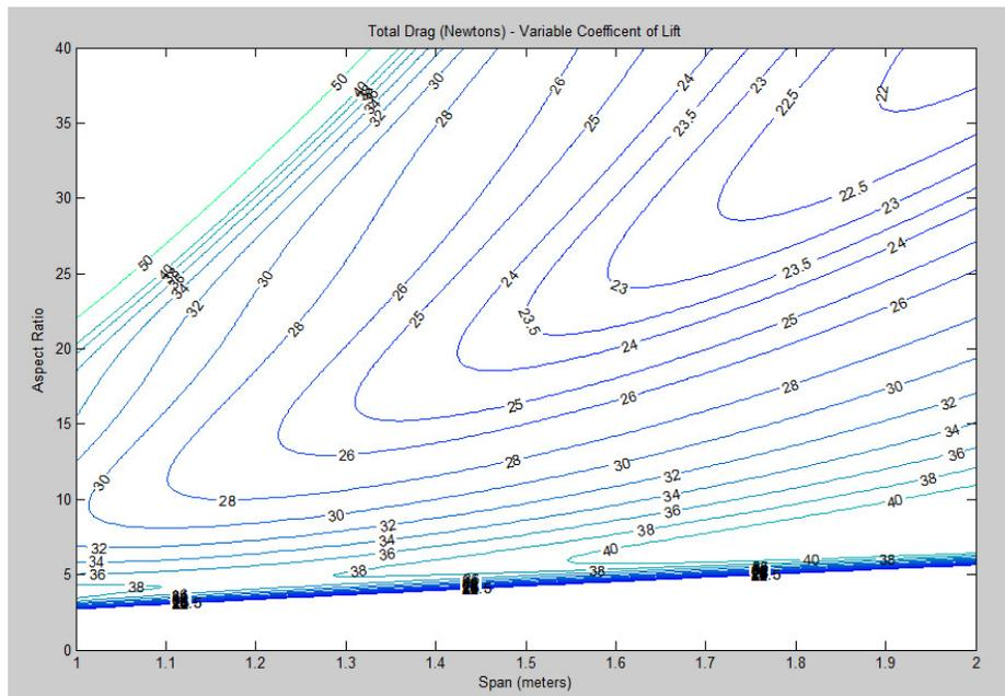
Figure 7 – Contour Plot of the Total Drag Force Developed By the Main Wing
