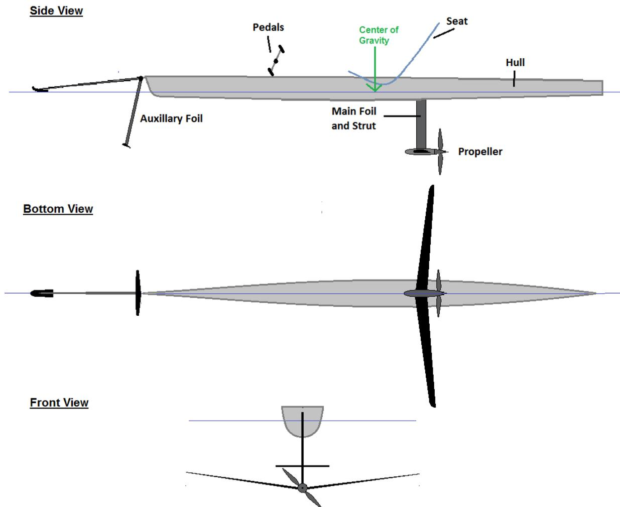
Figure 1. Vehicle Configuration Schematic
