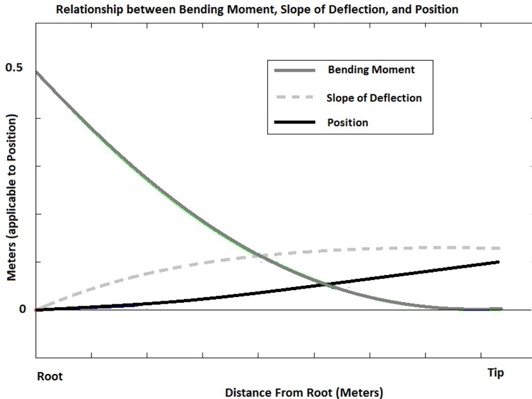
Figure 9 – Plot of the relationship between bending moment, slope of deflection, and position, and normalized tip displacement.
