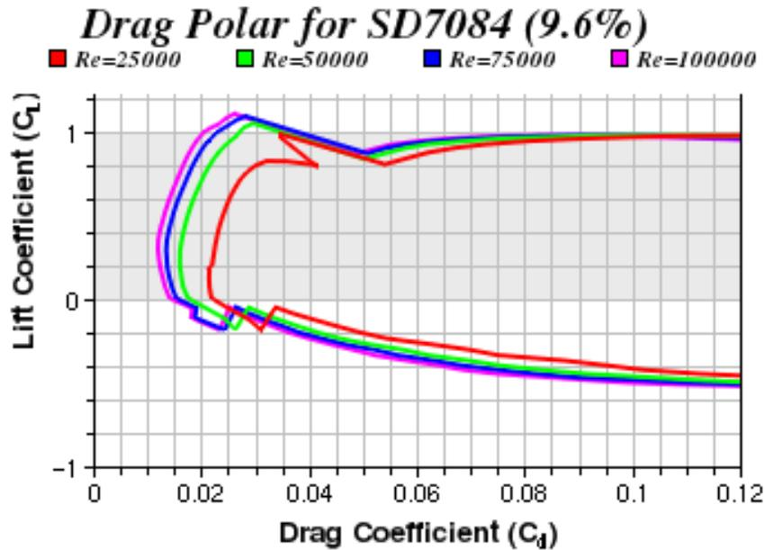
Figure 4. Plot of Coefficient of Lift to Coefficient of Drag at Different Reynolds Numbers<sup>16</sup>
