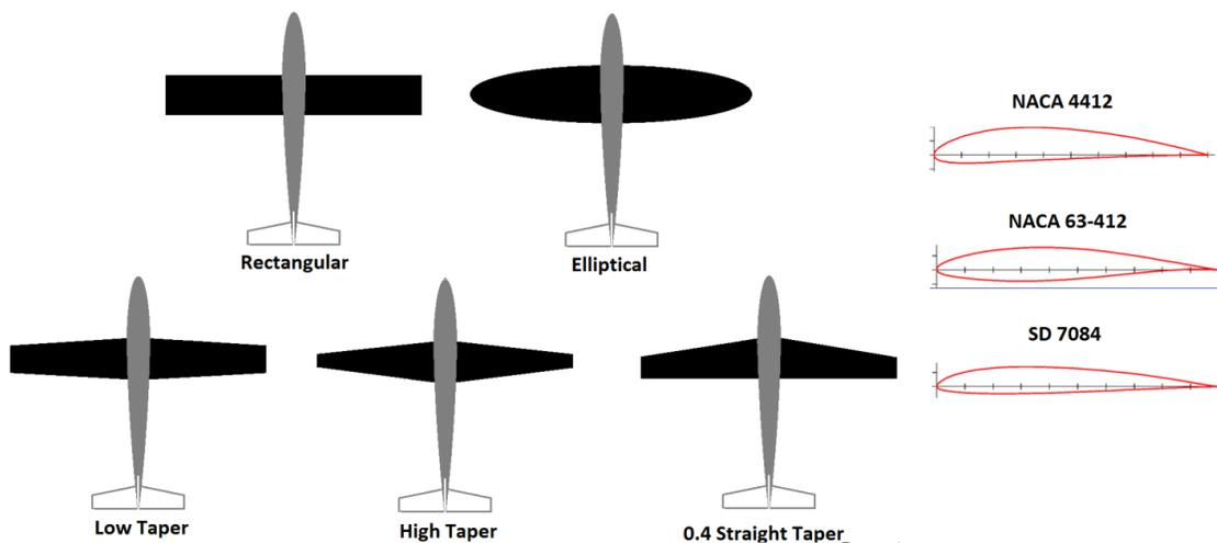
Figure 2. Wing Planform Shapes And Airfoil Section<sup>9</sup>
