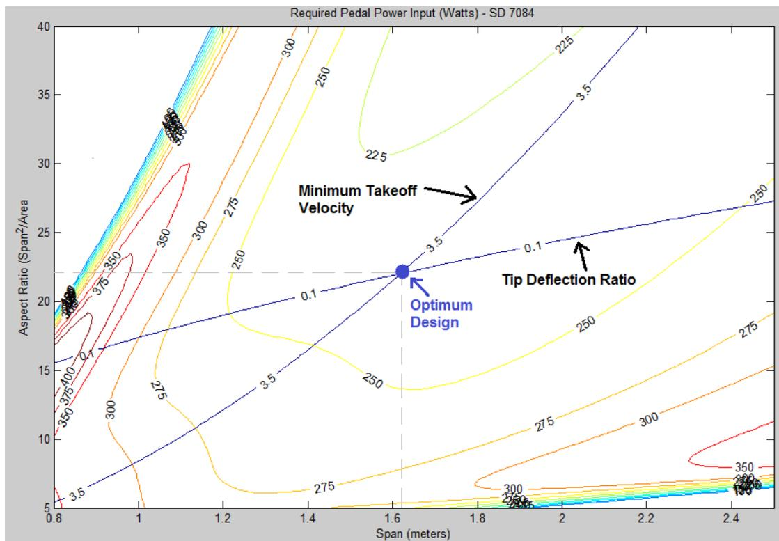
Figure 10. Graphical optimization relating contour plot of required power input, the normalized tip deflection ratio, and maximum takeoff velocity for a SD 7084 foil at design speed. (Normalized tip displacement ratio is the height of tip deflection divided by one half of total wingspan)
