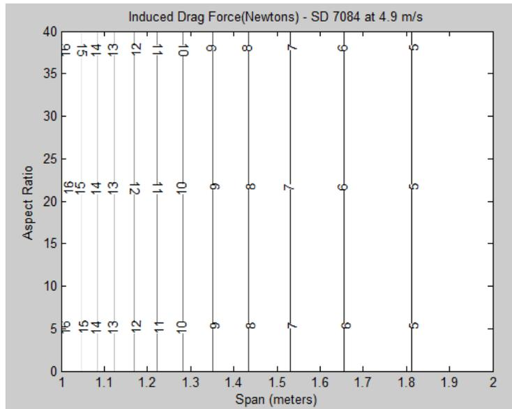
Figure 3. Contour Plot of Induced Drag (for a SD 7084 airfoil). Note, induced-drag is shown to be independent of aspect ratio as wing area varies simultaneously.
