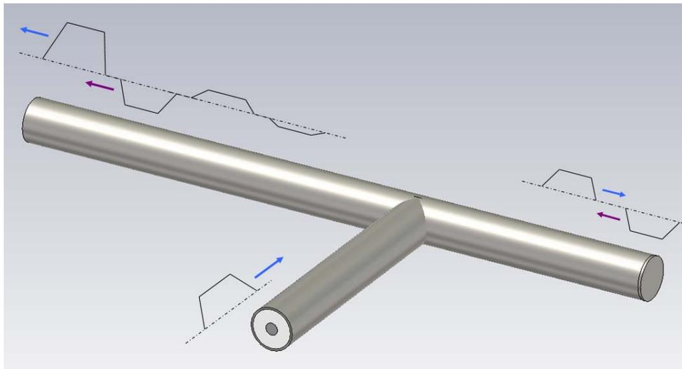
Figure 2: Tuning Stub CST Model
