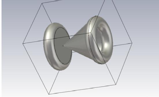
Figure 6: Discone Antenna in CST<sup>5</sup>
