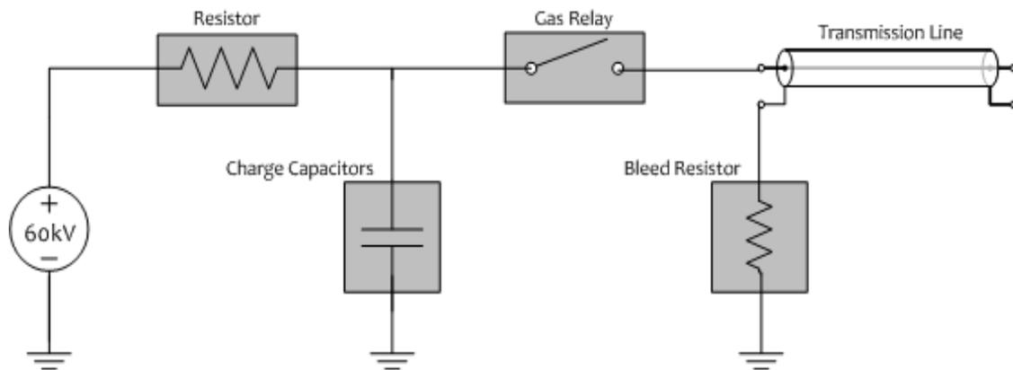
Figure 1: Low-Energy IEMI Schematic
