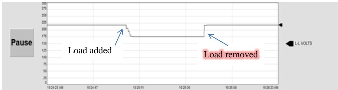
Figure 6: Loading with a resistive load of 1200 \Omega , voltage decreased from 220 V to 175 V
