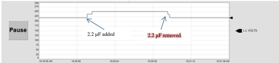
Figure 8: Loading with capacitive load; voltage increased from 220 V to 255 V
