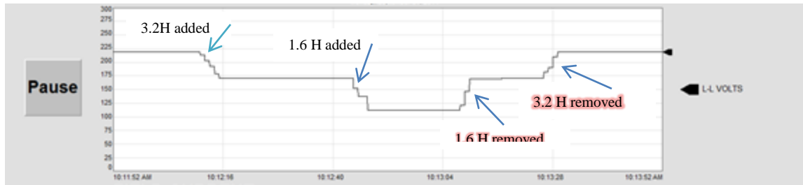
Figure 7: Adding inductive loads; voltage decreased from 220 V to 170 V to 110 V
