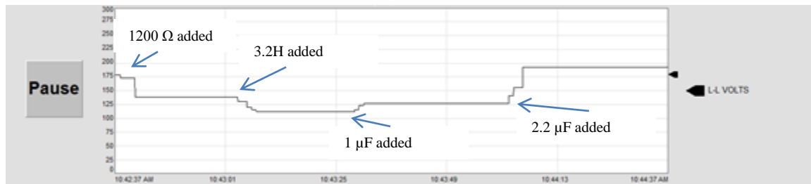
Figure 9: Loading with resistive → inductive → capacitive load in sequence; voltage changed from 180 V → 113 V → 190 V
