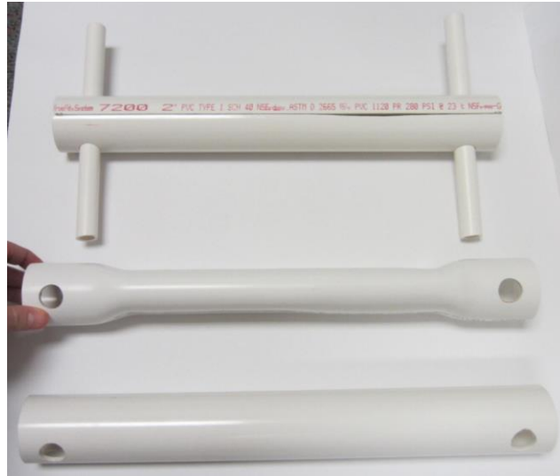
Figure 8. Cross-Section Effect on Torsional Rigidity
