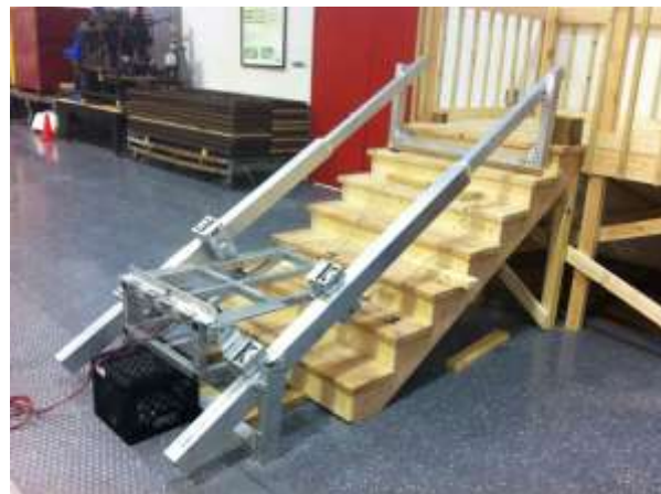
Figure 2 – The second iteration of the Wheelchair Escalator. Rendering images on top. Actual prototype on bottom.
