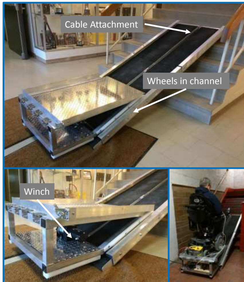
Figure 1 – Initial version of the Wheelchair Escalator, designed and manufactured by an intercollegiate team of ME students from UDM and Ohio Northern University. Photos courtesy of John Fernandez and Kathryn Skobrak.
