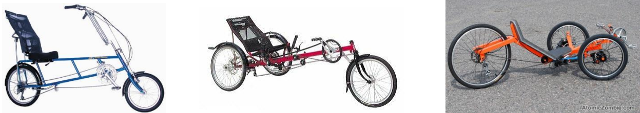
Figure 1: From Left to Right: A two wheeled recumbent bike 11 , a delta tricycle 12 , and a tadpole tricycle. 13
