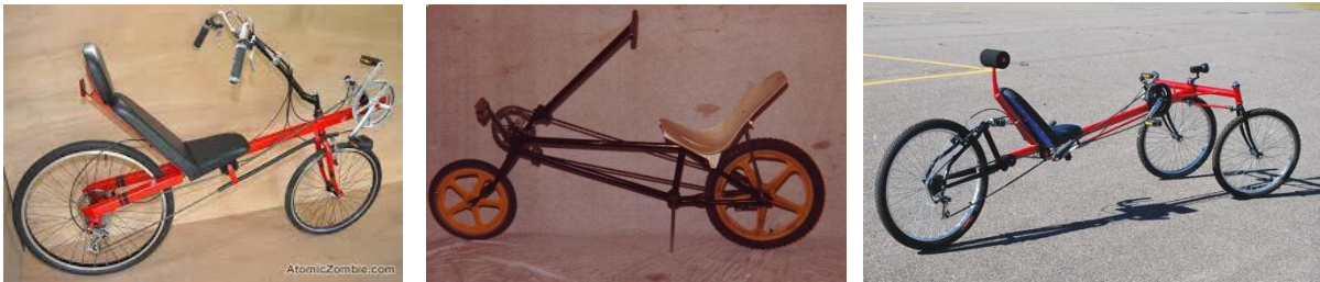
Figure 3: Three recumbent bicycles by increasing wheel base, including short wheel base, 16 medium wheel base, 17 and long wheel base. 18
