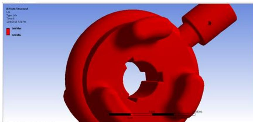
Figure 2 dog clutch FEA fatigue
