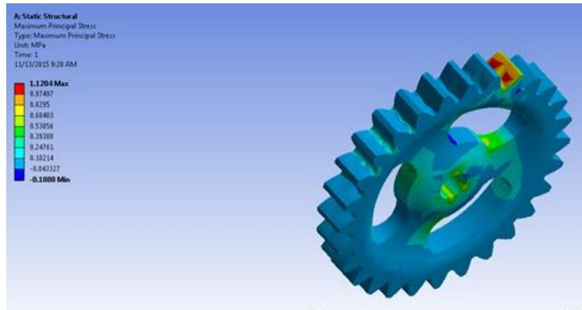
Figure 1 gear FEA Max Principal Stress
