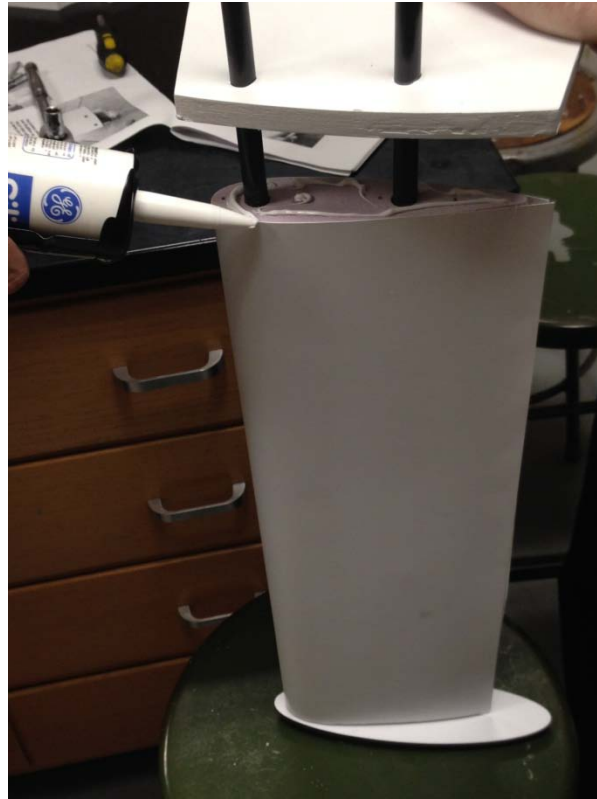
Figure (3): Caulking process of turbine rotor blade
